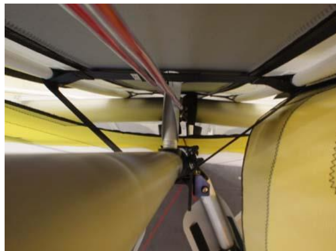
Figure 5-2 : Path of Tensioning Cables
