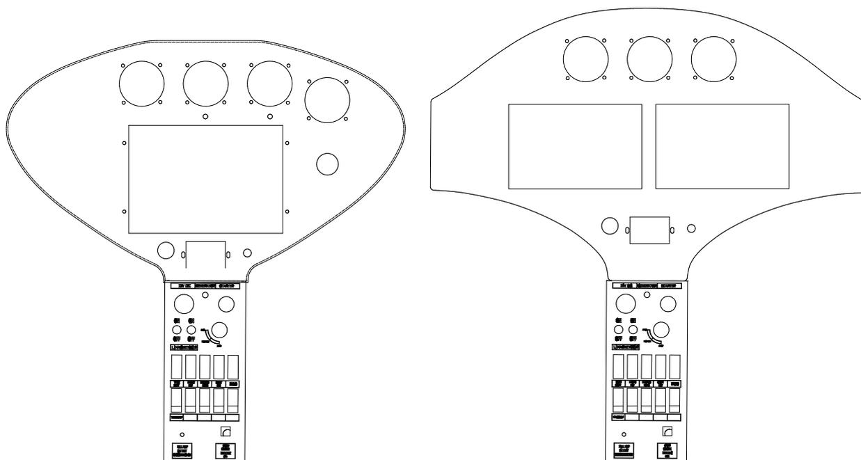
Small instrument panel (left) with Brauniger as the middle screen - Large instrument panel with two screen setup (Dynon D100 and EMS 120). Both are for illustration purpose only!
