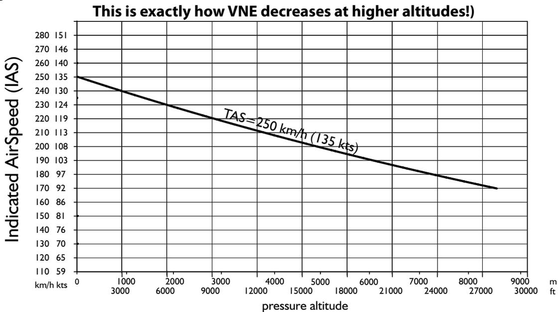
**WARNING!** Above pressure altitude of 4000 meters (13100 ft) VNE (see previous page) **MUST** be treated as True AirSpeed (TAS). Indicated AirSpeed (IAS) **MUST** be reduced accordingly! Table with IAS, TAS relation for 302 km/h (163 kts) is below:
