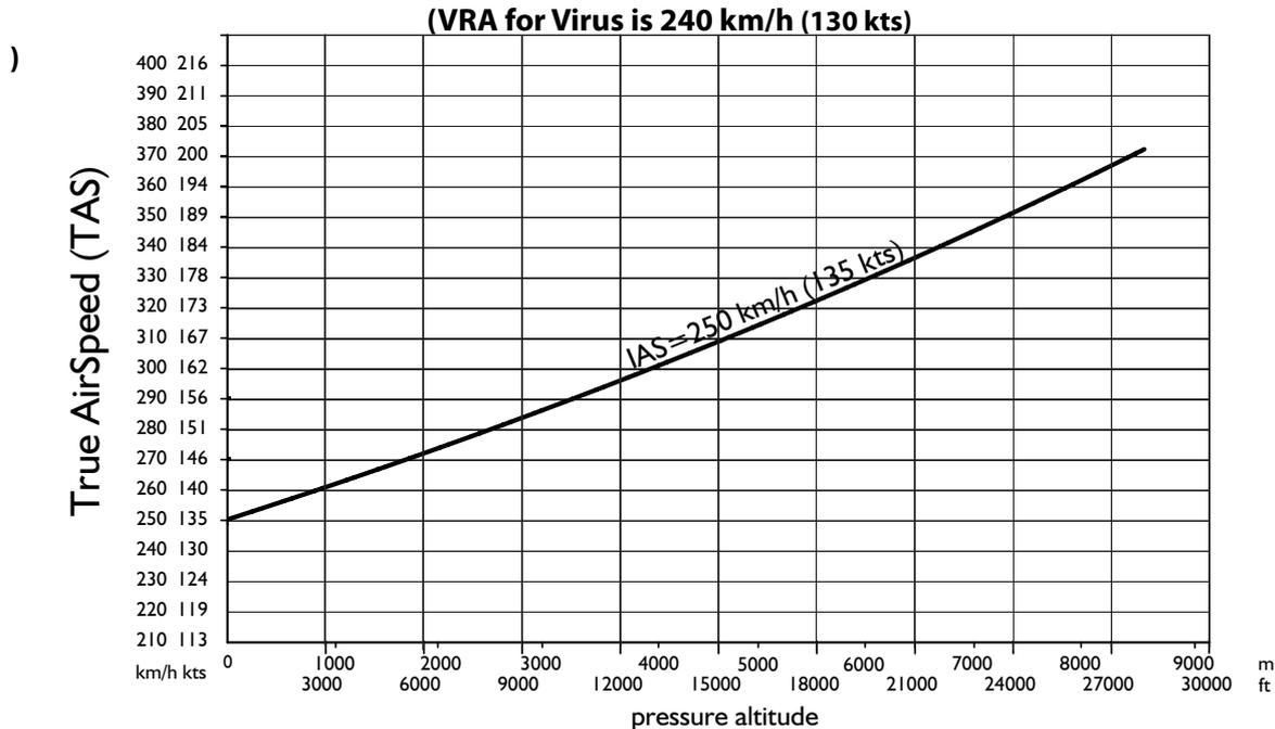
The graph below shows which indicated airspeed (IAS) must be maintained to keep the true airspeed (TAS) constant. Note that true airspeed (TAS) is constant along the entire servicable altitude range! (VRA for Virus is 240 km/h (130 kts) TAS).
