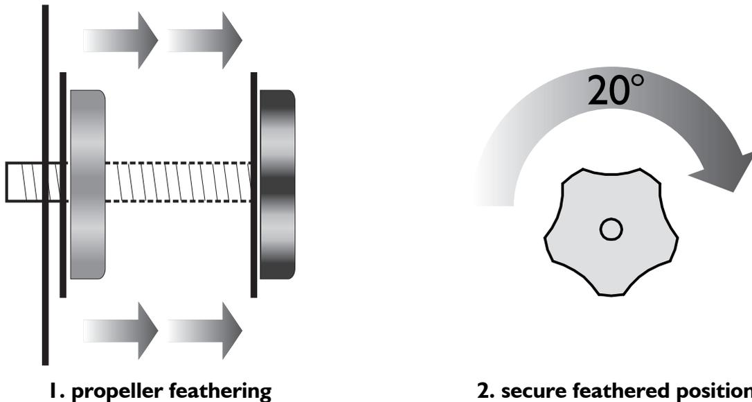
**WARNING!** Feather propeller only after the engine has stopped and at minimum pitch.
