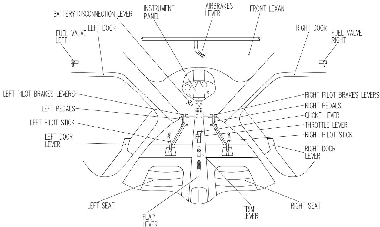
**Individual control levers:** pilot stick and rudder with belonging brake levers
