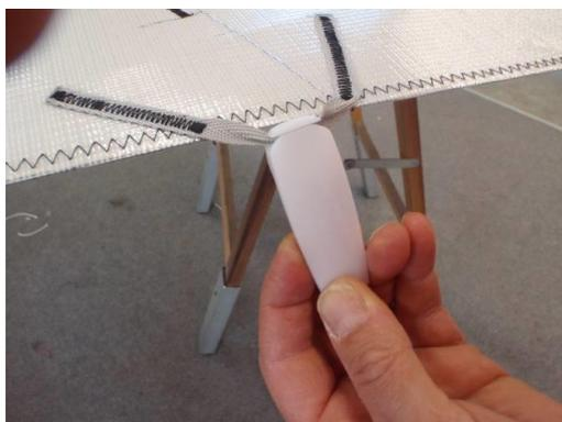
Figure 5-2 : Path of Tensioning Cables
